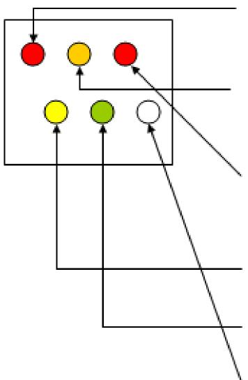
Upper left red light is function 1; controls water heater; when light is on, water heater is turned off
